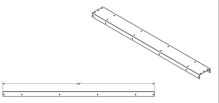
**TOLERANCE NOTES** TOLERANCES ON DIMENSIONS, UNLESS OTHERWISE NOTED ARE: SAWED, SHEARED AND GAS CUT EDGES (\$ 0,030") DRILLED AND GAS CUT HOLES (\$ 0,030") - NO CONING OF HOLES LASER CUT EDGES AND HOLES (\$ 0,010") - NO CONING OF HOLES BENDS ARE ± 1/2 DEGREE ALL OTHER MACHINING (± 0.030") ALL OTHER ASSEMBLY (± 0.060") PROPRIETARY NOTE:
